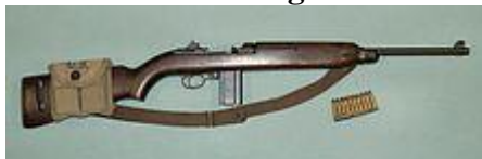
WW II M1 Carbine with a magazine pouch mounted on the stock that held two spare 15-round magazines
